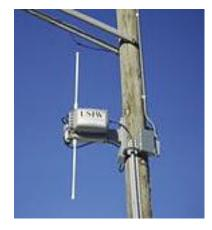
power (hence the habit of installing them on power and light utility poles). This "all radio" approach means that nodes must be within range of each other and form a contiguous pathway back to special aggregation nodes that have more traditional access to the Internet. Nodes then relay traffic, somewhat like a fire-bucket brigade.
